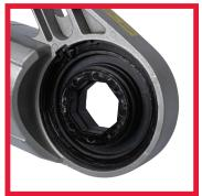
Portable Cyclone® is compatible with 11-R and 12-R die headed threaders.
