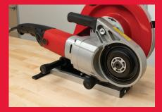
Pipe threader serves as the power source for bending.
